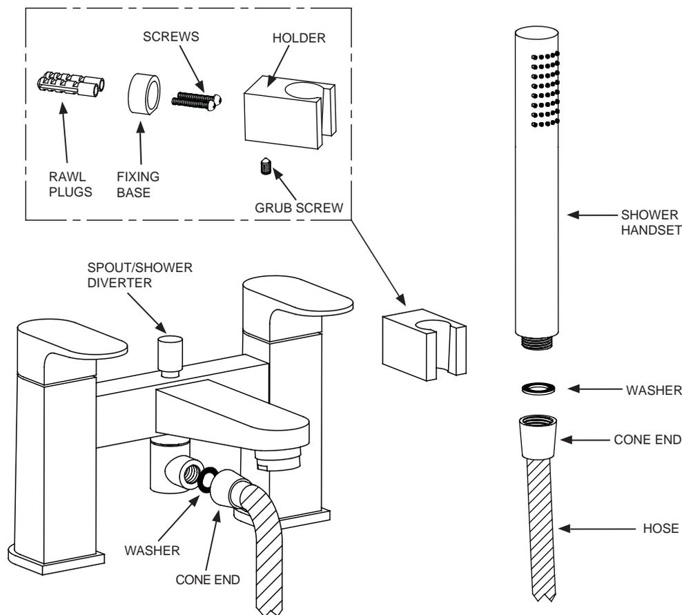
Insert a washer into the cone end of the hose and screw to the shower handset.
