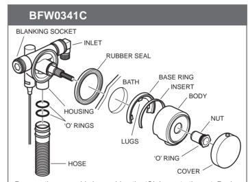
Prepare the assembly by pushing the 'O' ring onto the nut. Push the rubber seal onto the housing, and hold the unit in position from the outside of the bath. From the inside of the bath place the base ring over the bath hole, if the hole is to small, snap off one of the lugs with a pair of long nose pliers. Slide the insert and body into the base ring and screw on the nut, finally push on the cover.
