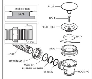
From below push the rubber seal into the hole in the bath (see detail), then push on the housing. From inside the bath place the plug hole in position on the seal, screw in the bolt and tighten (use the small bolt for bath thicknesses up to 9mm and the large bolt for thicknesses from 9mm to 35mm), finally screw in the plug.
