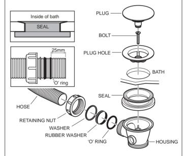
From below push the rubber seal into the hole in the bath (see detail), then push on the housing. From inside the bath place the plug hole in position on the seal, screw in the bolt and tighten (use the small bolt for bath thicknesses up to 9mm and the large bolt for thicknesses from 9mm to 35mm), finally screw in the plug.
