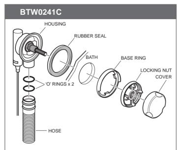
Push the rubber seal onto the housing, and hold the unit in position from the outside of the bath. From the inside of the bath place the base ring over the bath hole, screw on the locking nut, finally push the cover onto the splines of the housing. Insert the 2 'O' rings into the grooves on the inside of the hose and push the hose onto the housing.
