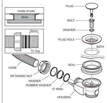
From below push the rubber seal into the hole in the bath (see detail), then push on the housing. From inside the bath place the plug hole in position on the seal, place the washer onto the bolt and screw in the housing (use the small bolt for bath thicknesses up to 9mm and the large bolt for thicknesses from 9mm to 35mm). Place the plug into the hole. To adjust the plug release the nut, screw/unscrew the bolt until the required position is obtained, re-tighten the nut.
