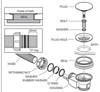
From below push the rubber seal into the hole in the bath (see detail), then push on the housing. From inside the bath place the plug hole in position on the seal, place the washer onto the bolt and screw in the housing (use the small bolt for bath thicknesses up to 9mm and the large bolt for thicknesses from 9mm to 35mm). Place the plug into the hole. To adjust the plug release the nut, screw/unscrew the bolt until the required position is obtained, re-tighten the nut.
