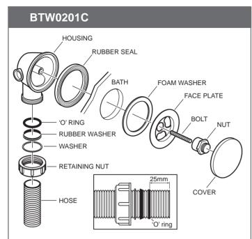
Push the rubber seal onto the housing, screw in the bolt and hold the unit in position from the outside of the bath. From the inside of the bath place the foam and face plate over the bath hole and screw on the nut, finally screw on the cover.
