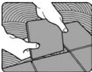
Now you can lay the floor tiles as normal. Remember to leave all adhesives to dry naturally, we recommend waiting for two weeks before turning the heating system on. If any tiles need to be taken up, for any reason, we recommend that extreme care is taken to avoid damaging the heating system.
