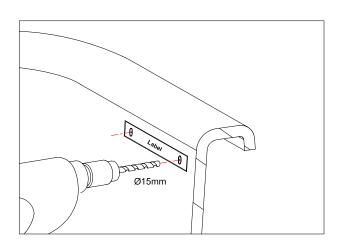
Drill the 4 holes using the template stuck on the bath.
