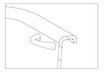
Tighten the nut using the wrench. Don't over tighten as this may cause damage to bath.
