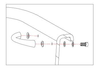
Remove the template, and install the bath grips to the bath.
