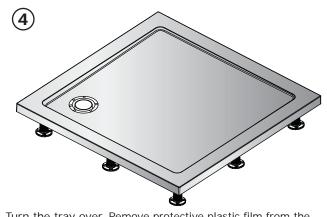
Turn the tray over. Remove protective plastic film from the areas near the waste and those sides of the tray which will be against a wall.
