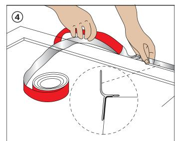
It is recommended that the 'easyseal' water sealing strip should be installed at the sides against wall. For the detailed installation method,
