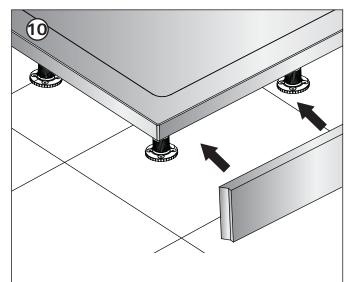
First fix the rebated panel pushing it firmly on to the panel clips. Then fix the remaining panel in the same manner.
