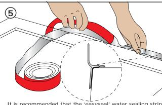
It is recommended that the 'easyseal' water sealing strip should be installed at the sides against wall. For the detailed installation method,
