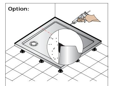
\* If the 'easyseal' water sealing strip is not installed, please seal joints between tray and wall with an anti fungal silicone sealant and allow to set.
