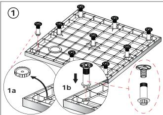
Turn the tray over and use the cardboard packaging as a protective mat. Remove the green caps, and insert the feet to the indicated positions.
