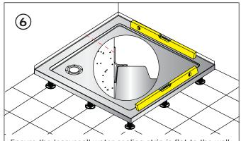
Ensure the 'easyseal' water sealing strip is flat to the wall. Place the tray into position and level both ways using the legs. After the tray has been levelled adjust all the inner feet to stabilise the tray. When level fix these legs to the floor with silicon sealant or 'no more nails' type adhesive.
