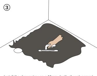
Install the shower tray on a 15mm depth of weak cement mix (sand/cement ratio 5:1). Tile adhesive can be used as an alternate to sand or cement.
