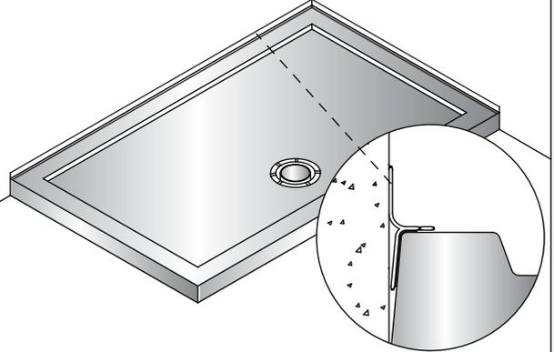
Ensure the 'easyseal' water sealing strip is flat to the wall. Place the shower tray onto the cement bed and apply gentle pressure with the palm of the hand to bed the tray into position.
