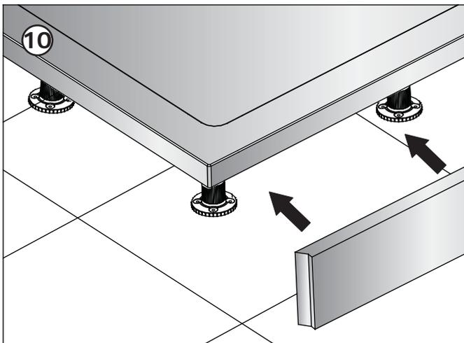
First fix the rebated panel pushing it firmly on to the panel clips. Then fix the remaining panel in the same manner.
