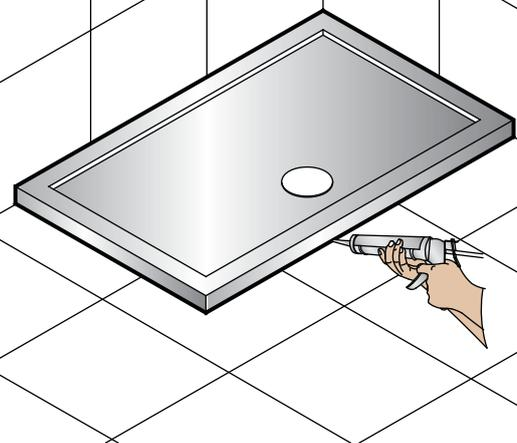
Tile and seal joints with an anti fungal silicone sealant and allow to set.
