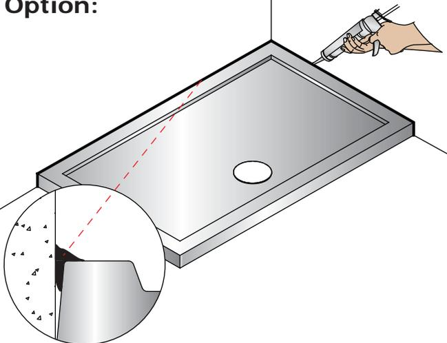
\* If the 'easyseal' water sealing strip is not installed, please seal joints between tray and wall with an anti fungal silicone sealant and allow to set.
