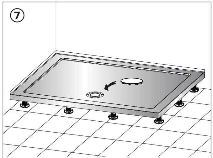
When shower tray is set remove the remainder of the protective plastic film and connect the waste pipe and check for leakage.
