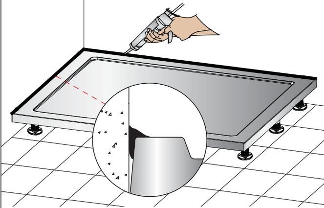
\* If the 'easyseal' water sealing strip is not installed, please seal joints between tray and wall with an anti fungal silicone sealant and allow to set.
