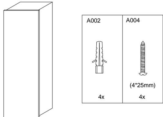
Insert the wall plugs provided into the holes, reposition the cabinet and screw securely into place.
